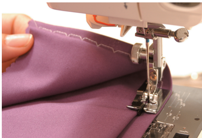
A blind hem is easy when you use a blind hem foot
